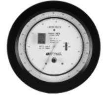
Series 1000 gauges have capsules up to and including the 150 psig range and Bourdon tubes in the higher ranges. Pressure is applied to the capsule or Bourdon tube through a single case connection. Readings are referenced to atmospheric pressure in the case. Available in 26 standard ranges, (including vacuum and compound ranges) Series 1000 Gauges combine aneroid convenience with precision-liquid-column accuracy. They are compact, yet readability is excellent.
